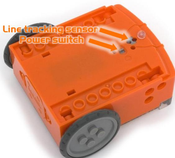
Edison's line tracking sensor is made up of two parts: a red LED light and a light sensor.
