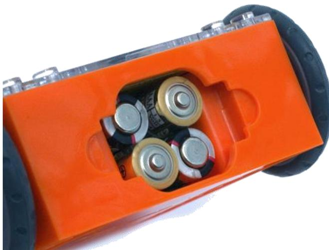
Ensure the batteries are in the right way.
